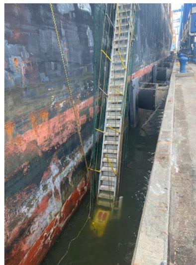
**Example: The member alerted the vessel that the gangway was not safely footed on the pier. While re-positioning the hoist line parted, causing the gangway to fall into the water. Vigilant review before allowing employees access, prevented a potential injury event.**
