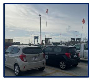
We installed bicycle flags that fly higher than 8 ft (typical container height) so that the Sparks and other vehicles can be
